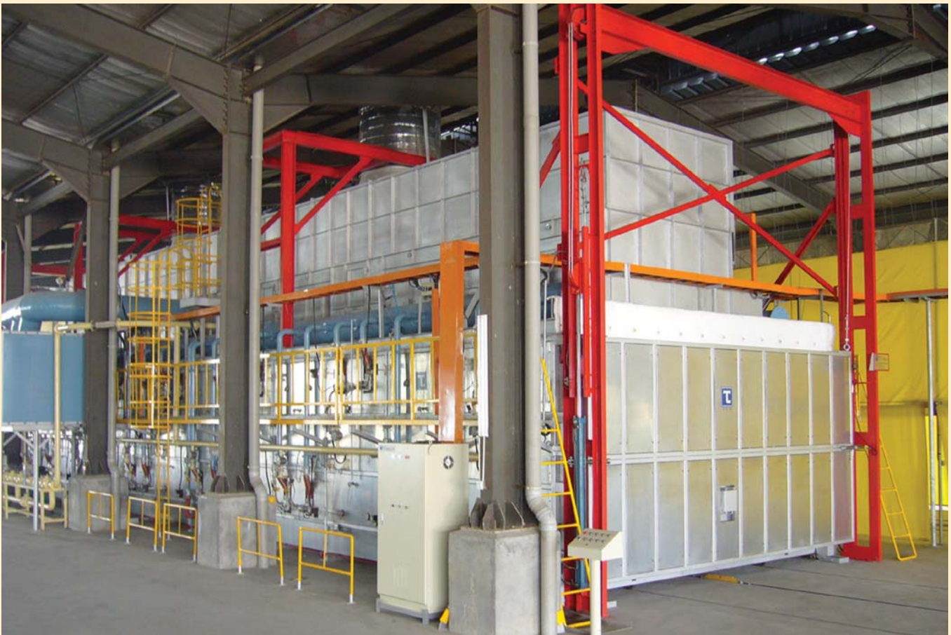
160 cubic meter capacity Shuttle kiln
